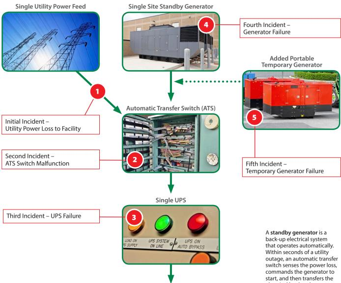
An Automatic Transfer Switch (ATS) is often installed where a standby generator is located, so that the generator may provide temporary electrical power if the utility source fails. This switch acts as an interconnection between the various power sources in a redundant power system. It is deemed to be a critical component at the Marysville data centre.
