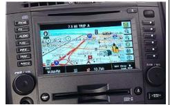
and interactive driver interface equipment to enable planning and detailed route guidance based on static, stored information. Information is stored in a Geographic Information System (GIS) that analyses, stores, and displays both spatial and non-spatial data.
