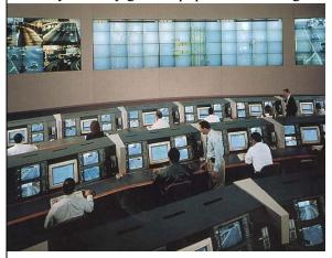
communication system, which connects the camera to a control centre. The primary objective of a CCTV camera is to provide surveillance of freeway / highway segments or intersections and visual confirmation of incidents, however it may also be used to detect incidents. A secondary benefit is the monitoring of environmental conditions including precipitation and visibility. CCTV supports other applications including vehicle classification and enforcement.
