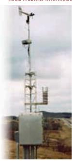
Road Weather Information Systems (RWIS) provide detailed roadside weather conditions and road surface temperature data through the use of in-road and roadside sensors. A complete RWIS combines the roadside data readings with standard meteorological data to provide precise road weather forecast and pavement condition predictions for up to 12 hours. This information is used by road maintenance providers as a tool to plan winter maintenance activities.
