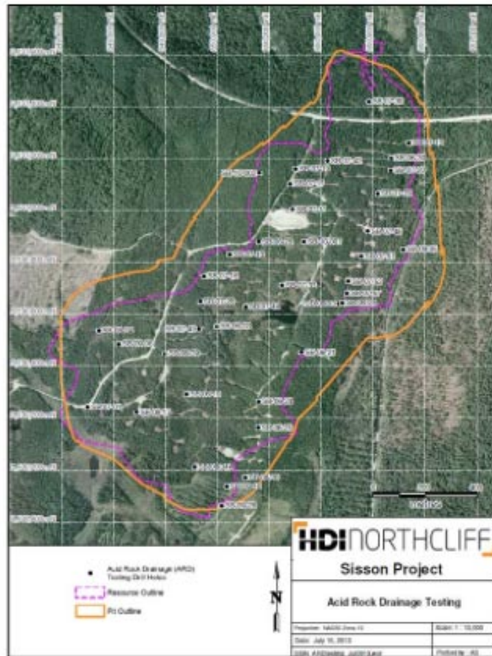
Figure 5: Proposed mining area and location of drill hole collars used for ML/ARD characterization studies (Source: Northcliff).
