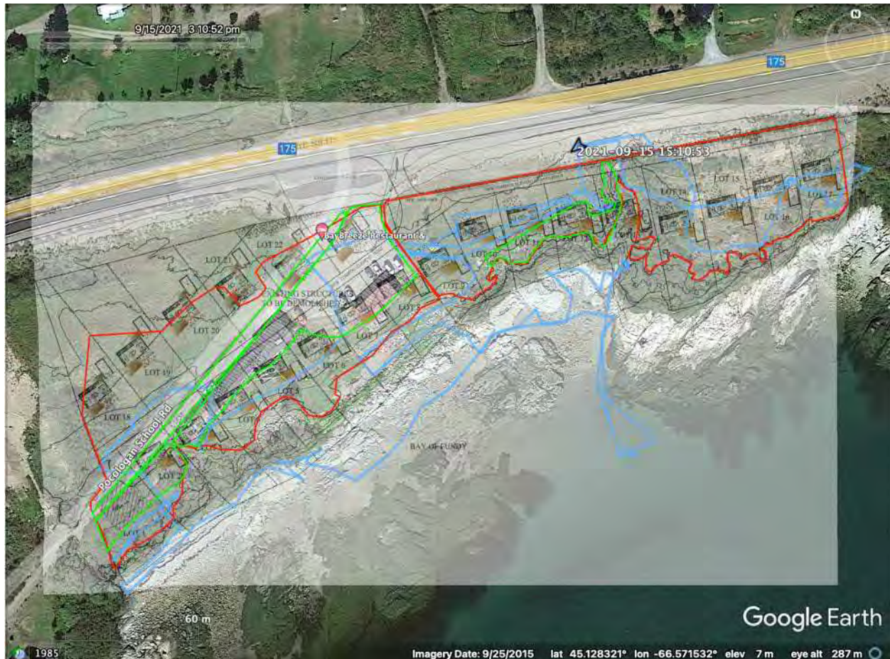
Figure 48. Mitigation model for project development area (PDA), if construction plans include sub-surface disturbance. Red outline is 50 m buffer zone, requiring 5 m testing grid for Standard Test Pits (STPs). PDA is in east and west sections. Blue line is surface inspection GPS tracks. Green lines enclose areas where test excavation is not feasible/warranted: old road = 1061 sq m; fill SW = 425 sq m; restaurant and parking lot = 1721 sq m, total 3207 sq m. Pocologan West = 6391 sq m; Pocologan East = 5412 m; Total = 11,803 – 3207 = 8596 sq m testable on 5 m grid. 8596 sq m divided by 25 sq m (5 m x 5 m grid unit) = 343 STPs plus about 7 on 10 m grid = 350 STPs total estimate.
