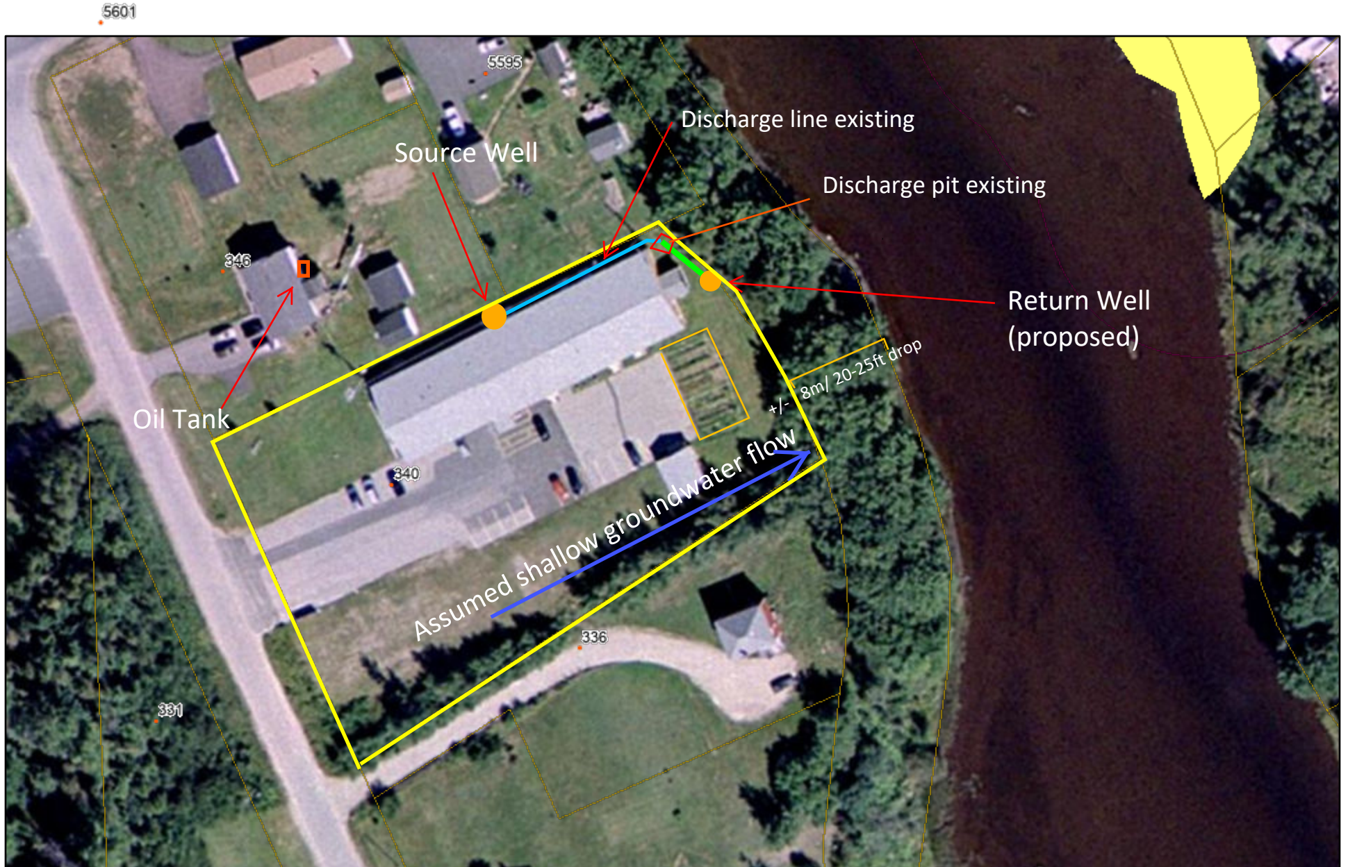
Figure 3 - Site layout with Source and Return Wells
