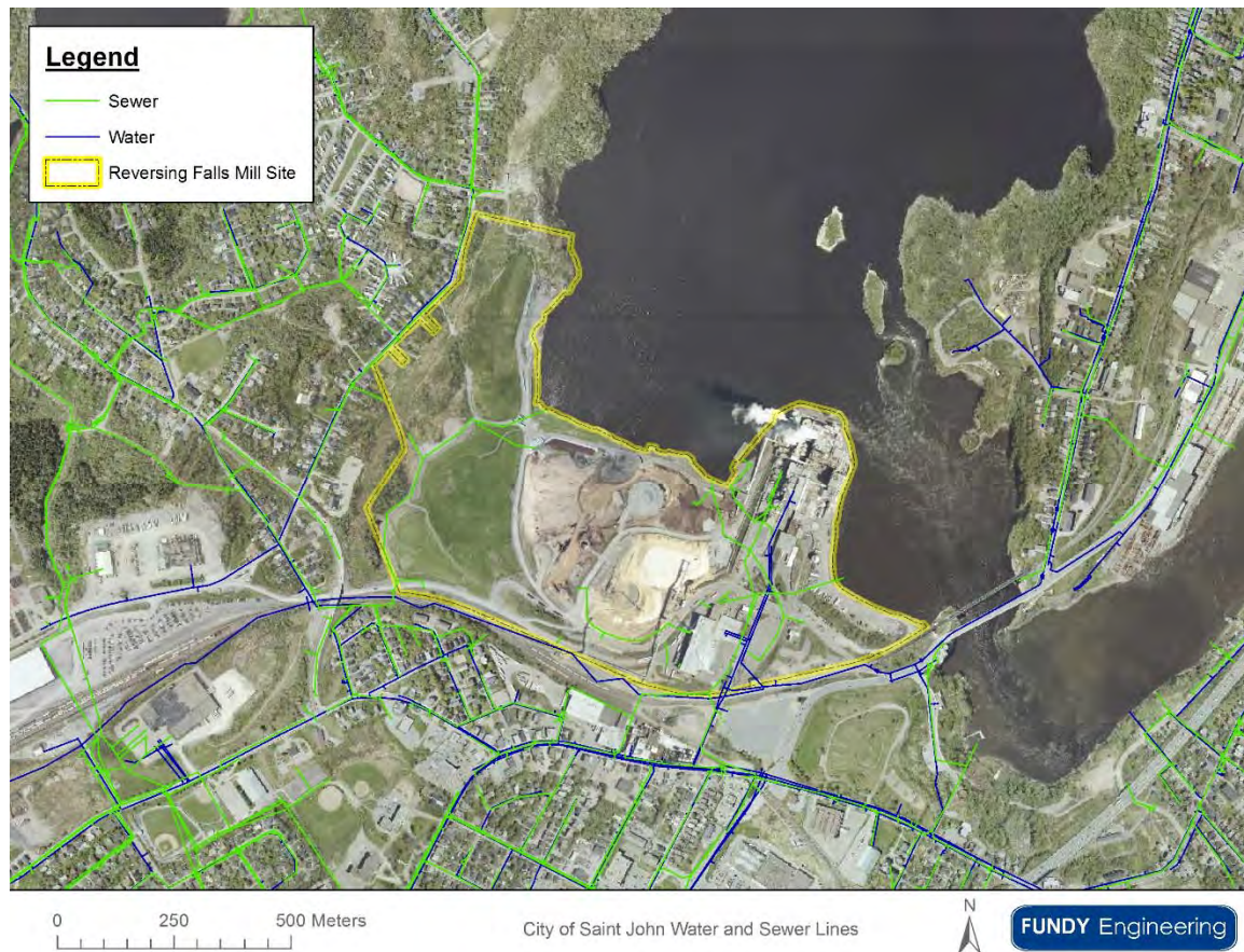
Figure 54. Aerial photograph, circa 2014, showing the major waterlines and sewer lines in the vicinity of the Reversing Falls Mill in Saint John, New Brunswick.
