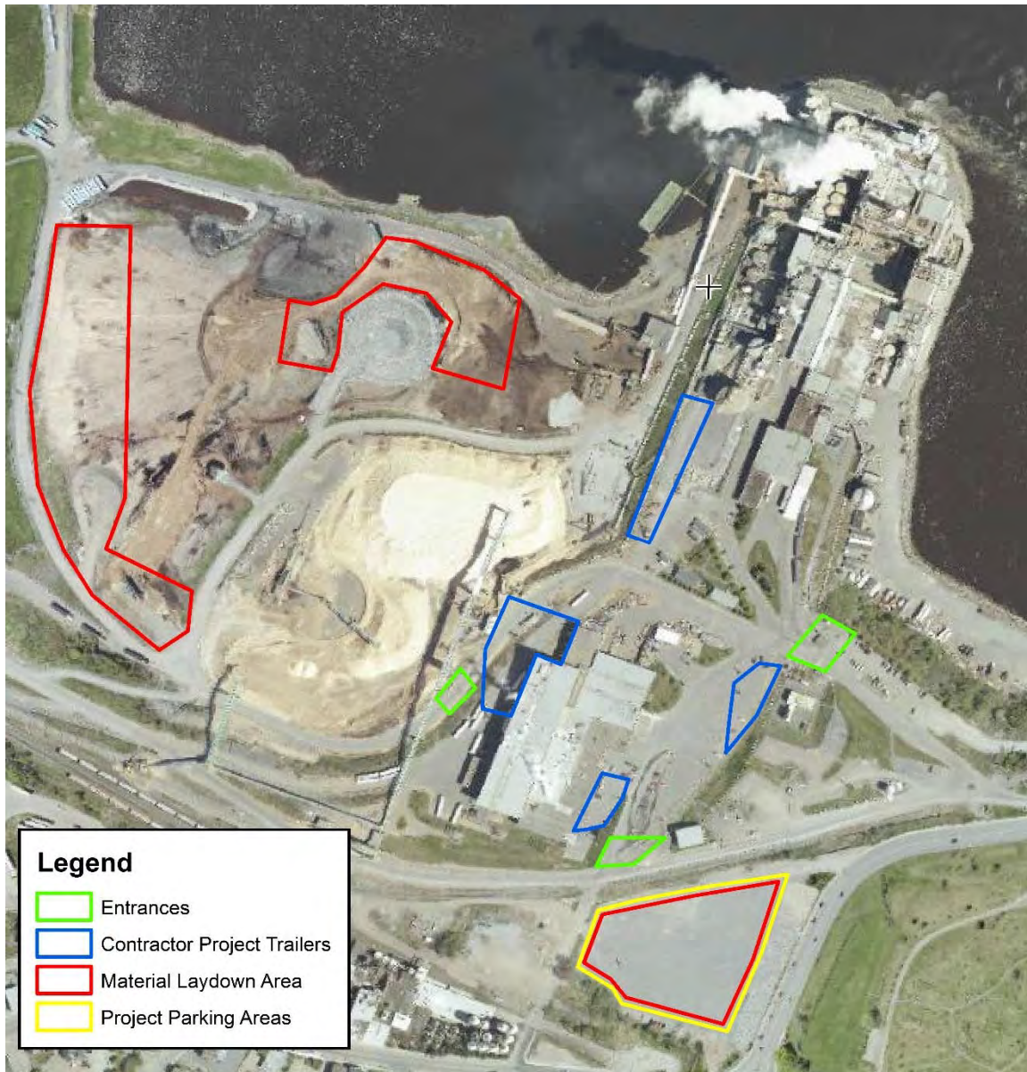
Figure 16. Aerial photograph of the Reversing Falls Mill in Saint John, New Brunswick showing the locations proposed for contractor project trailers, project parking areas, material laydown areas, and construction entrances for construction of the pulp dryer modernization project.
