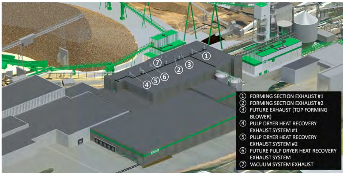
Figure 13. Three-dimensional model showing the exhaust points on the roof of the pulp dryer building proposed for the Reversing Falls Mill in Saint John, New Brunswick.
