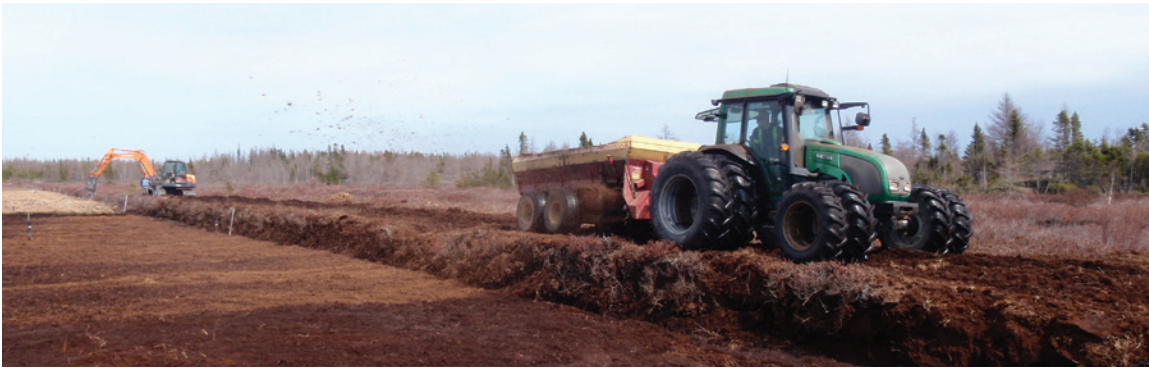
Figure 5. V-shaped side-discharge spreader.
