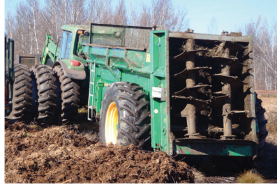
Figure 4. Apron box manure spreader with vertical beaters.
