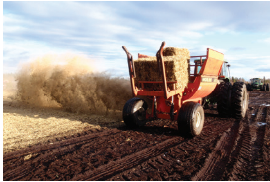
Figure 9. Side-discharge mulcher (rear view).
