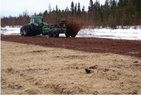
Figure 3. Plant material being spread using a hydraulic push (hydro-push) manure spreader with horizontal beaters.
