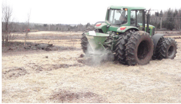
Figure 11. Fertilizer being applied with a conical spreader hooked up to the tractor's PTO.
