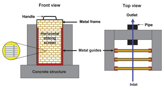
Note: Wherever the screens may be installed, you have to make sure the screen panels fit snugly in the metal guides. Therefore, it is important to fix the metal guides on both sides and bottom of the concrete structure.
