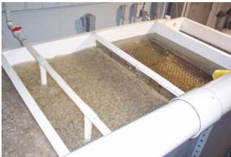
Figure 21: Moving bed biofilter with Kaldness media.
