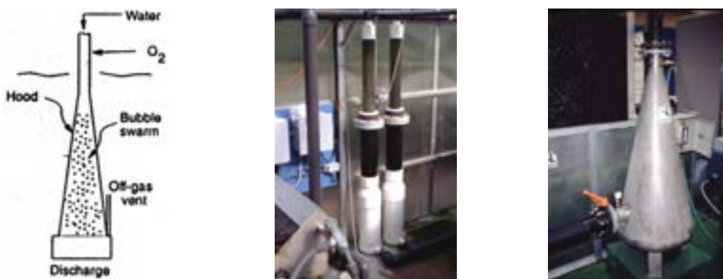
Figure 26: Process flow diagram and photos of Oxygen Saturators
