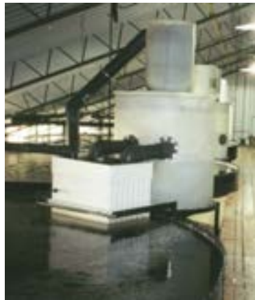
Figure 23: Down-flow micro-bead plastic media biofiltration. (L: Home-made biofilter – R: Holder-Timmons Engineering biofilter)
