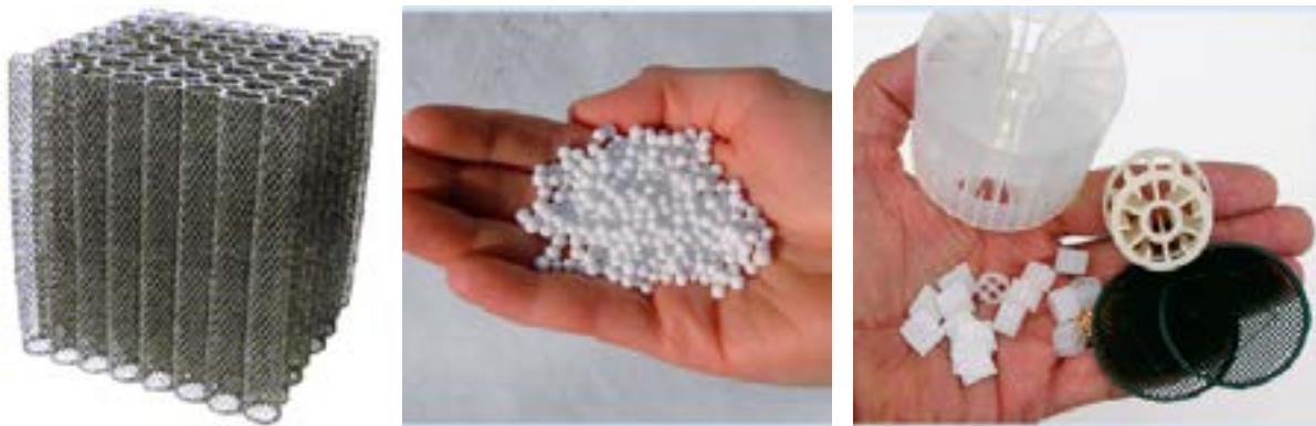
Figure 20: Some examples of biofilter media. Left - BioBloc Centre - Polystyrene beads Right - Random dump engineered media
