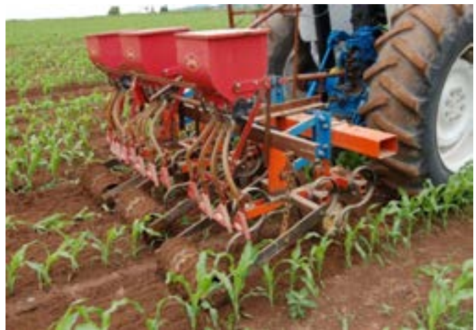
Specialized inter-planter (photo provided by the New Brunswick Soil and Crop Improvement Association)
