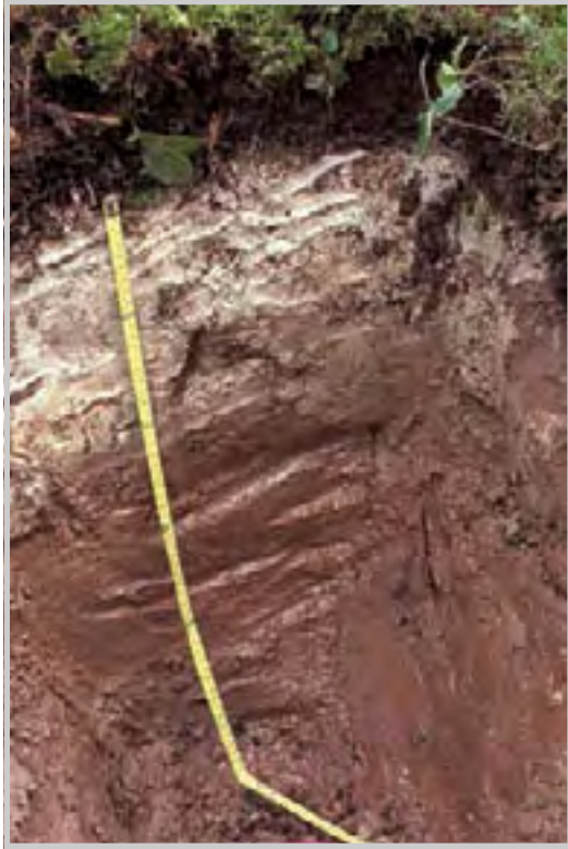
The Castaway Ecodistrict is underlain by clay loam subsoils of low permeability such as the one pictured here. Forest productivity is low overall, except where very gentle slopes contribute to improved drainage.
