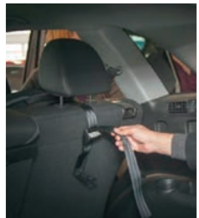
Always attach the top tether to the anchor point for that seat.
