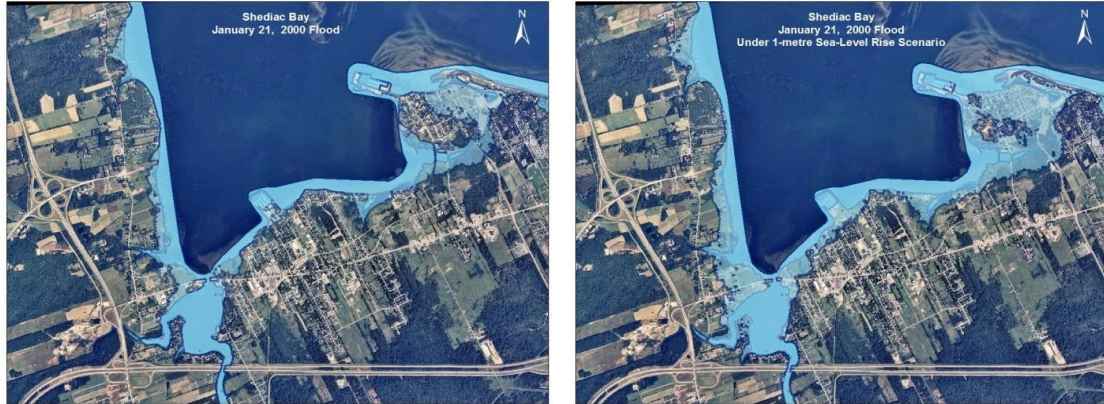
Figure 1. LiDAR-derived maps showing the January 21, 2000 flooding event (left) and the same event (right) given a sea-level rise scenario of one metre on an orthophoto (geometrically corrected aerial photo) background map.
