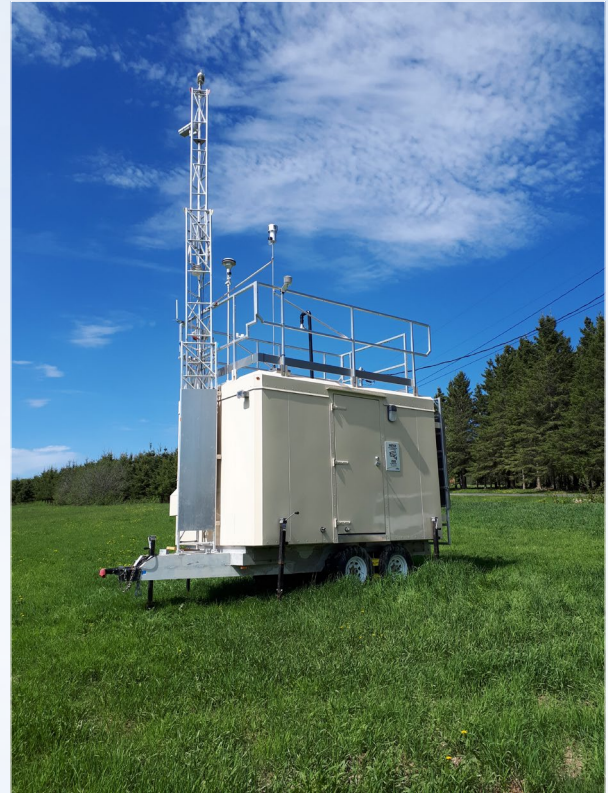
DELG's mobile air quality monitoring unit.
