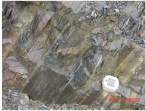
Stop 31 - Medium to dark grey, thin-bedded calcareous siltstone and minor calcilutite (brown-weathered).
